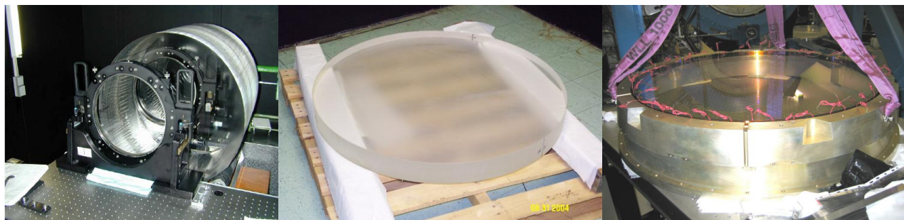
Figure 6: a) The merged infrasil blank (605x550mm) undergoing homogeneity testing at Heraeus. b) The flowed out 1m blank at Corning prior to shipping to Sagem for polishing. c) The final 950x80mm cryostat window mounted in its cell ready for wiring up of the heater circuit.
